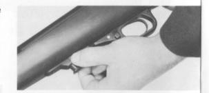
press the trigger. The rifle is now unloaded and the firing pin floating free.
