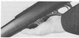
Do not forget to release the cocking lever when a round is being chambered.
