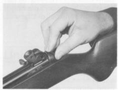
Press the trigger assembly into its recess until the catch engages.
