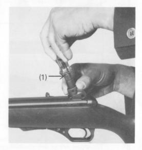
HK elevation adjustment device for adjusting the rifle.
