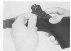
Press the bolt bushing inward with your thumb pushing upwards at the same time; this allows the bushing to slide out of position.
