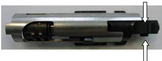
Insert the two pushrods into the receiver.
