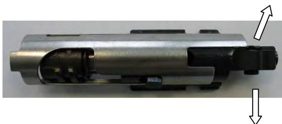
Remove the firing pin.
