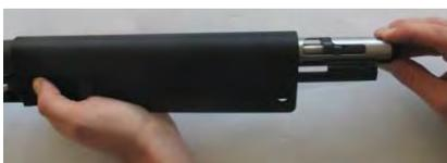
Locate the cocking lever into the recess and pull it fully back in its slot.
