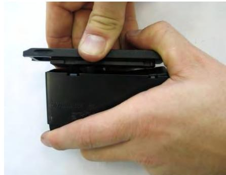
Ensure that the button of the locking plate latches into the magazine floor plate.
