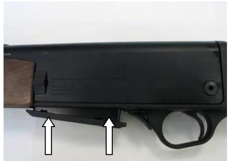
Pull the bolt fully back using the cocking lever. Release the cocking lever. When the cocking lever is released, a round will be fed from the magazine into the chamber.
