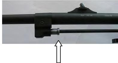
First remove the rear bolt in the receiver.
