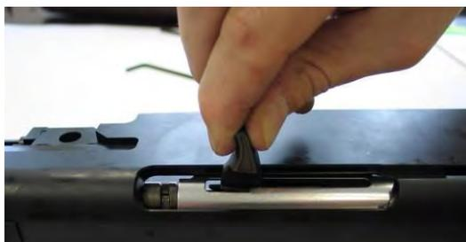
Insert the pushrods on both sides of the drive unit and secure them with the clips.
