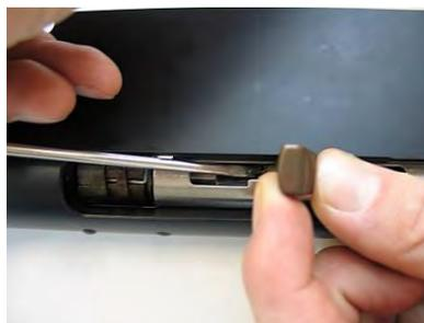
Remove the bolt assembly with the push rods from the receiver.
