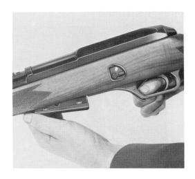
Remove the magazine by pressing the magazine catch. Retract cocking lever quickly, tilting the rifle somewhat to the side to permit a round that might be left in the chamber to slide out of the ejection port into your hand. Close the rifle and pull the trigger. The rifle is now unloaded and uncocked.
