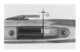
the bolt head carrier. You can determine this, if you can put a sheet of paper between bolt and bolt head (see fig., gap >0). If this gap has disappeared, please have the weapon checked by your local gun dealer as this technical condition would cause excessive strong recoil forces and thus damage the bolt system.
