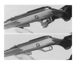
Then retract the bolt all the way by means of the cocking lever on the right side of the rifle. The catch lever located behind the cocking lever will engage and hold the bolt open. Depressing the catch lever slightly will cause the bolt to snap forward, chamber a round from the magazine, and lock into the receiver. The rifle is now
