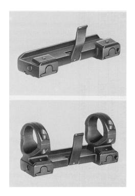
Our HK05 clamp mount readily accepts all standard telescopic sights. Should you wish to use an aluminum rail-type telescopic sight, loosen the two hexagon socket screws on the bottom of the 05 clamp mount, slide on the telescopic sight and tighten the two hexagon socket screws firmly at the rails. If you are using a steel telescopic sight, please also use the retaining rings.
