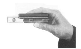
Rotate the bolt head clockwise one quarterturn, and then remove it from the locking piece. Finally, remove locking piece, firing pin and firing pin spring from the bolt head carrier by rotating the locking piece further
